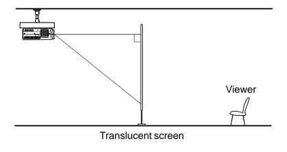
Perform the "Projection mode" setting on the menu screen for the projection method. 51>
